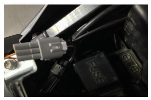
The connection from the Suzuki vehicles to your AVDI is established by connecting the 6 pin connector to a DB9 connector and then to a DB25 connector in order for the signal to enter the DB25 connector on the AVDI via the following table:
